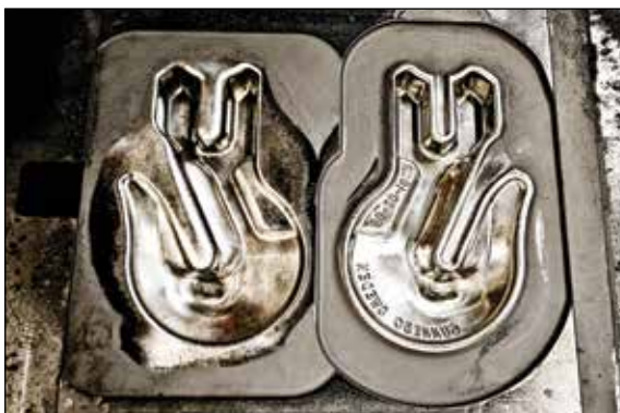
Forging die (left) for producing hooks (right). Courtesy: Gunnebo Industries, Sweden.
