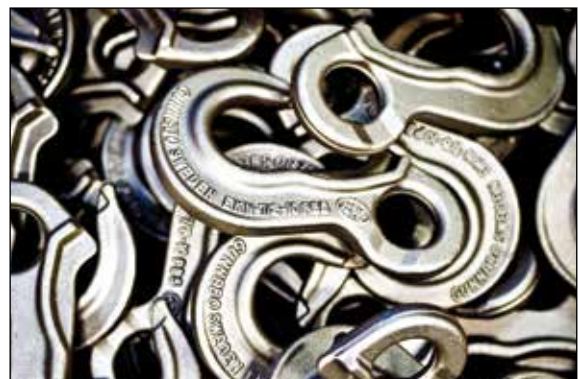
Forging die (left) for producing hooks (right). Courtesy: Gunnebo Industries, Sweden.
